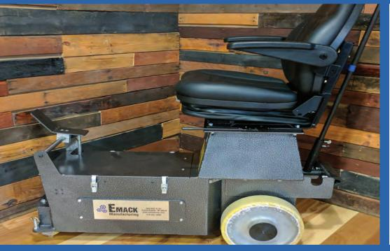
Aimed at helping industry professionals increase efficiency while reducing effort, the EMack Ryder Cart allows users to operate up to three sanders simultaneously, reducing sanding time and removing strain on the body. Single phase and 3-phase are available for 230V or 480V of power. For more information or to order, visit www.emackmfg.com or call 616.241.3040.
